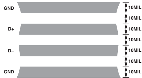
Figure 4. Arrangement of Signal Tracks
